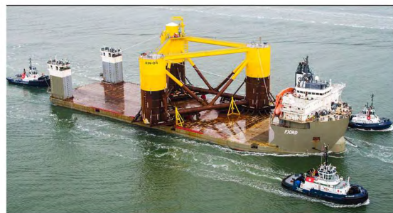
Figure 3 – Semi-submersible heavy lift vessel
