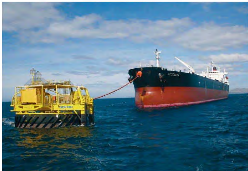
Figure 4: Single-point mooring buoy example.
