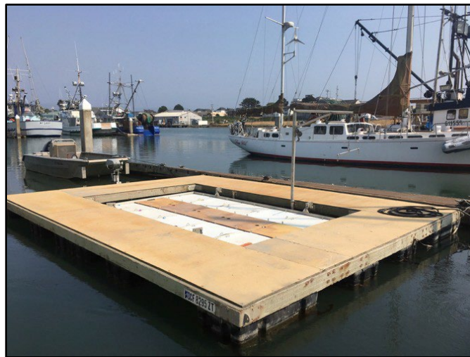
Figure 3. HBOC's floating upwelling system operated at Woodley Island Marina, Eureka, CA.
