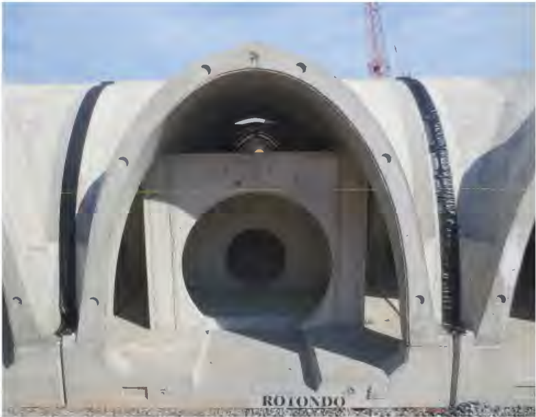
Internal outlet control structure installed at factory
