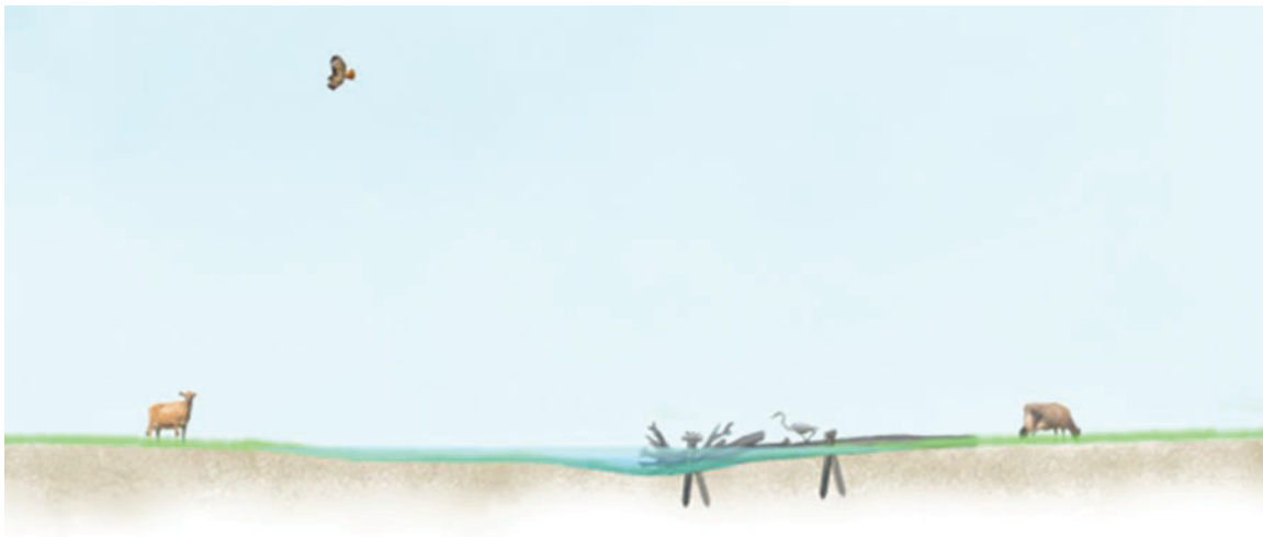
Figure 2-14. Floodplain channel through agricultural grasslands during flood flows in the Elk River. The low flow channel, set within a broad shallow floodplain channel, provides deeper flow paths with cover for fish to pass through agricultural grasslands to reach higher quality habitats as high water recedes. During dry periods, the floodplain channel is grazed.
