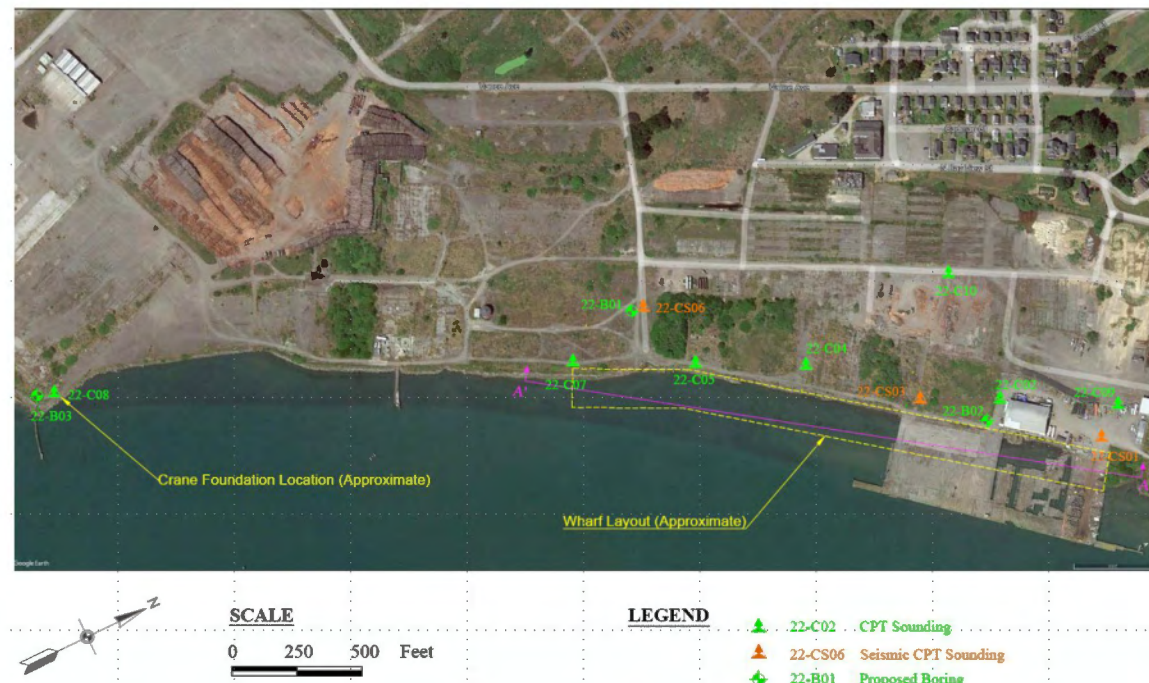
FIGURE 6-1: CPT AND DRILLED BORING LOCATIONS
