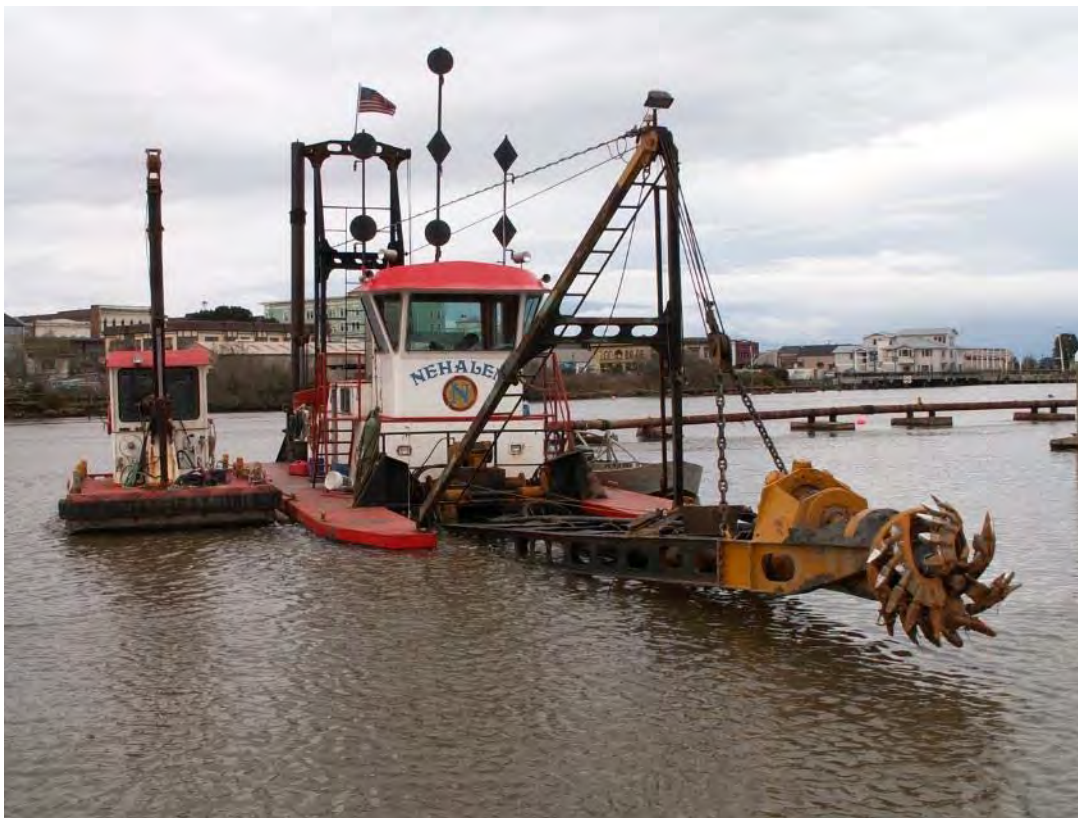
Figure 6. Cutterhead suction dredge, workboat, and floating pipeline (behind dredge) to be used for the Project.
