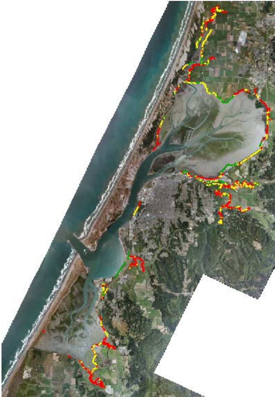
Figure 1. Diked and railroad shoreline vulnerability rating for Humboldt Bay; red-high, yellow-moderate, and green-low.
