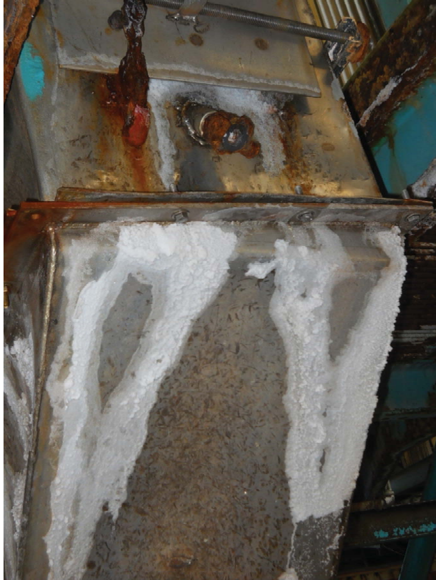
Oxidation and mineral precipitation of metal surfaces in AOI-1 Black Liquor Process and Recovery Area.
