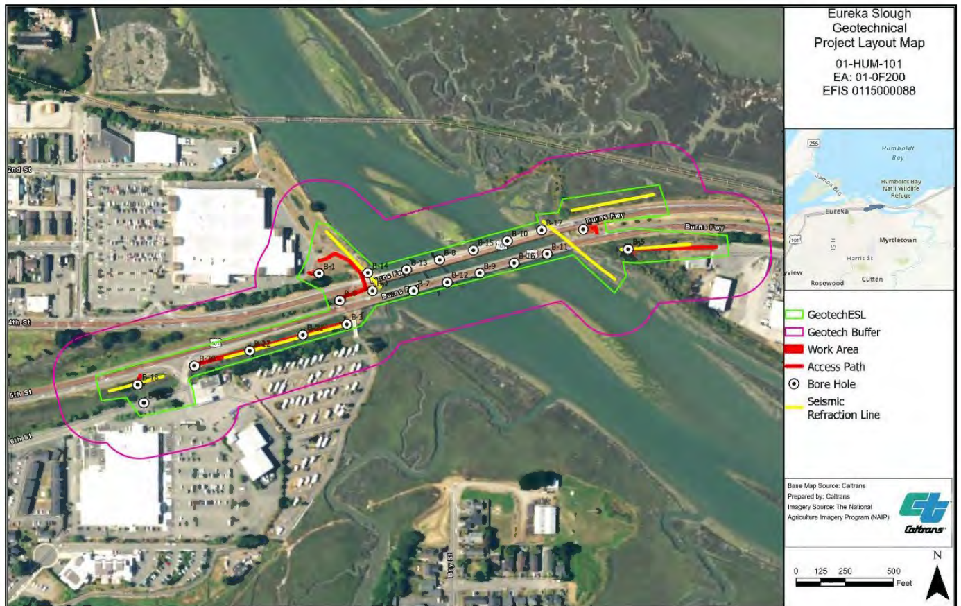
Figure 1. Eureka Slough Geotechnical Project Layout Map
