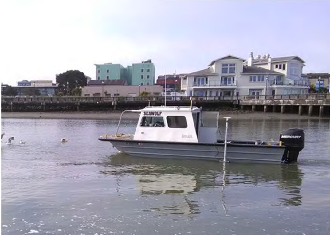
Figure 2. The TGAEC survey vessel Seawolf used for the sidescan sonar survey.
