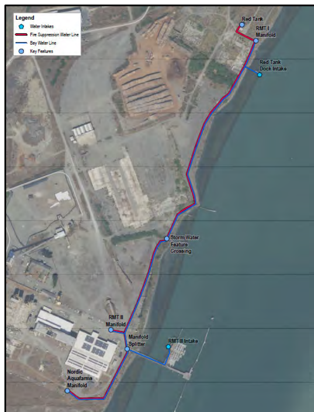
Figure 2: Location of bay water intakes, bay water piping and industrial water piping.
