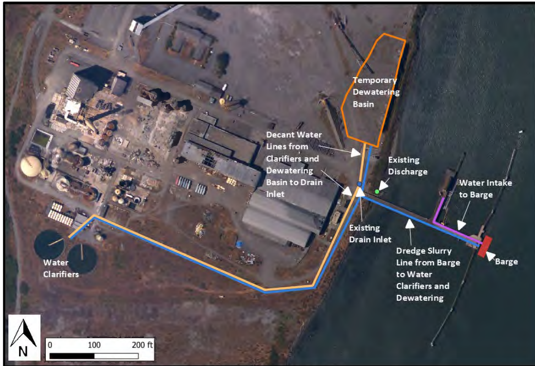
Figure 1. Configuration of currently permitted dredged material offloading and dewatering.
